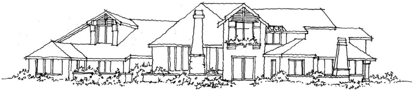
GABLES, DORMERS AND OTHER SMALLER ROOF ELEMENTS SHOULD BE PROPORTIONAL TO THE SPACES THEY COVER
